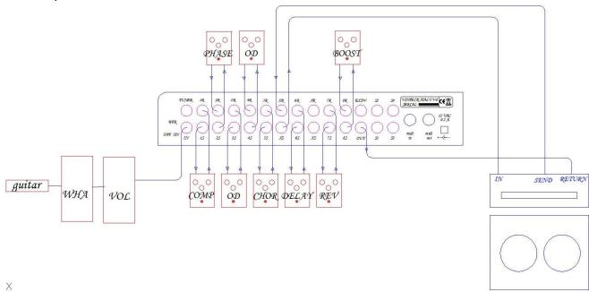
**Example 3**V-8 with 6 pedals in front, 2 pedals in send/return and volume in send/return before delays
